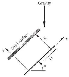
(a)The velocity distribution in the liquid layer
