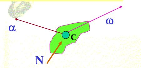
Mass Distribution: The Inertia Tensor of an object describes the object's mass distribution (a generalization of the scalar moment of inertia). Relative to a frame {A} is expressed as:
